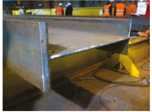
Fig. 21: Weld seam preparation for a welded butt joint of hot-rolled wide-flange beams for a composite bridge
