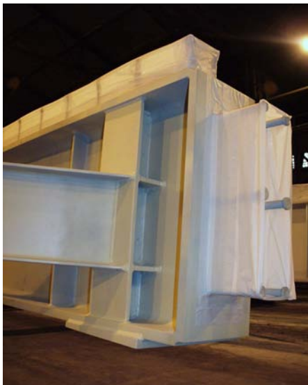
Fig. 6: Execution of detail of an I cross-beam welded onto a T-rib; left: a practical example during fabrication; right: execution with the required drainage openings
