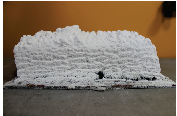
Fig. 6: When exposed to fire, fire protection coatings form an insulating carbonaceous char that delays the heating up of the steel structural component.
