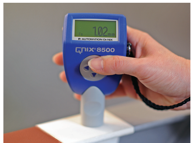
Fig. 15: Non-destructive measurement of the dry film thickness is conducted with the aid of electromagnetic gauges.
