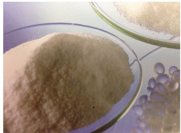
Fig. 5: Non-noxious ammonium polyphosphates are among the substances intumescent coatings are based on.
