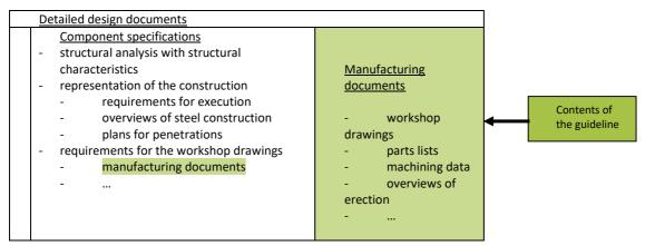
The manufacturing documents have to be written in such a way that those participating in the manufacturing are provided with the necessary information and technical requirements for the steel construction to be erected. In particular, the manufacturing documents must contain the data that form the basis for
